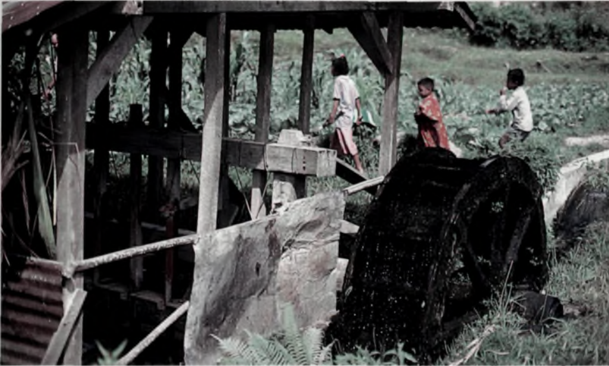
Water wheel powering a rice threshing machine in Sumatra, Indonesia.
