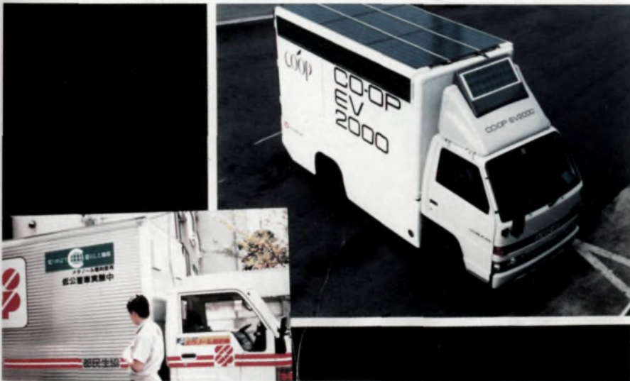
The Japanese consumer co-ops are carrying out field tests on electric and methanol cars to replace the diesel trucks currently being used. The electric car is on the right and the methanol car on the left.
