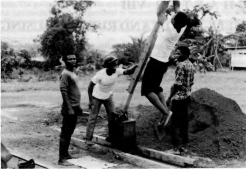
Project in Tema, Ghana: This Cinva Ram block-making machine can easily be used in self-help schemes Foto: CHF
