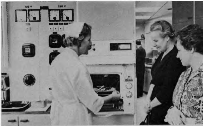
Housewives are always interested in the tests - Here an oven-fast dish is being tested in a special thermostatically controlled oven
