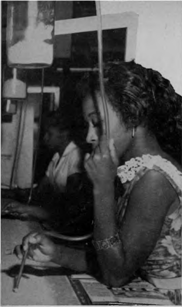
Discoloured rice is rejected and the sound grain is sucked into a jar above the sorter's head
