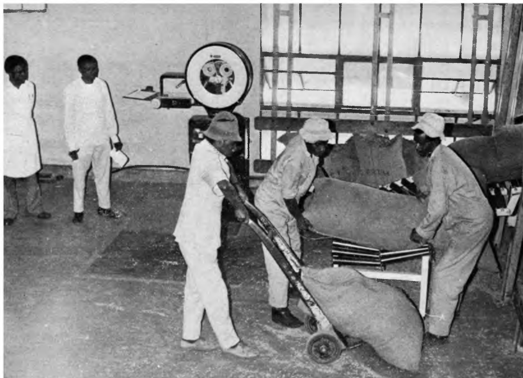
Sacks of coffee being received on the second floor of the Storage Building of KPCU before being emptied into bins ready for processing
