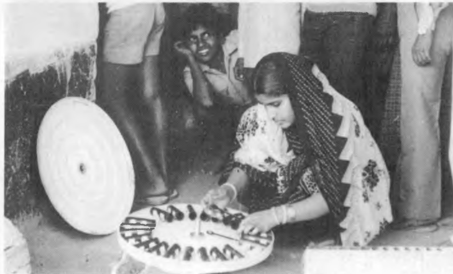
An employee of the Co-op Society taking out Gerber tubes from the centrifuge
