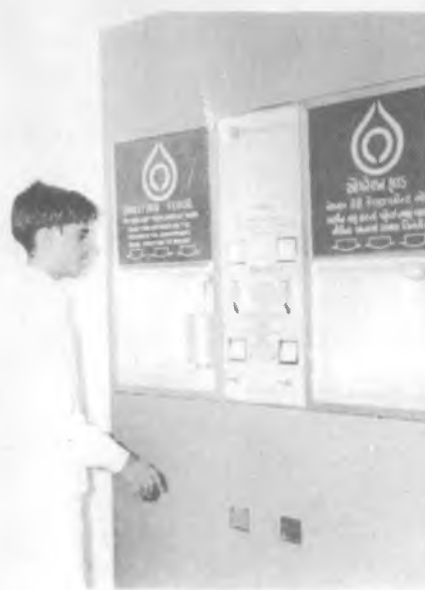
Bulk vending unit for dispensing pasteurized chilled milk into owners' containers.
