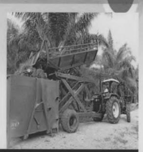
Mechanical High lift scissor trailer were raised up for directly loading the bunches into the Bin.
