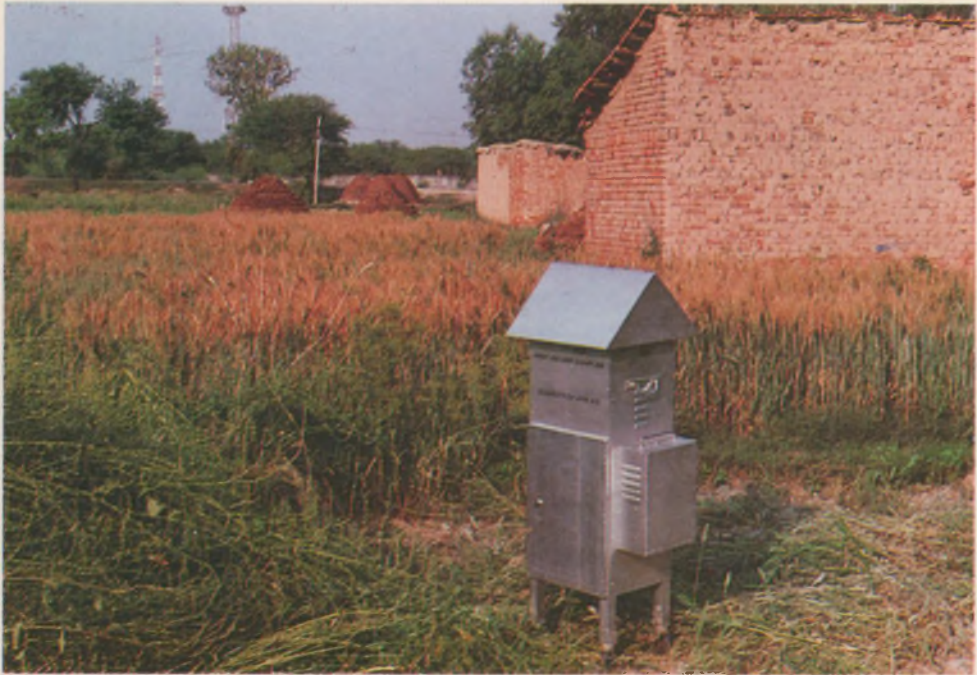
Air pollution : High volume air sampler installed at one of the plants of IFFCO in India
