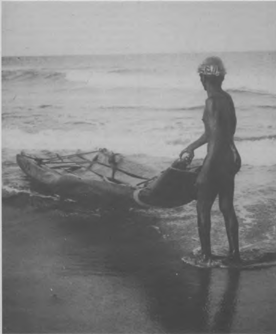
Catamarans, collapsible fishing craft, have been famous on India's Coromandel coast, near Madras, for centuries. A cross between a raft and a boat, the catamaran is made up of logs loosely held together with ropes. When not in use, the logs are untied and left to dry on the sand. Modern progress has come to the fisherman in the picture in only one form – a cellophane covering for the head.
