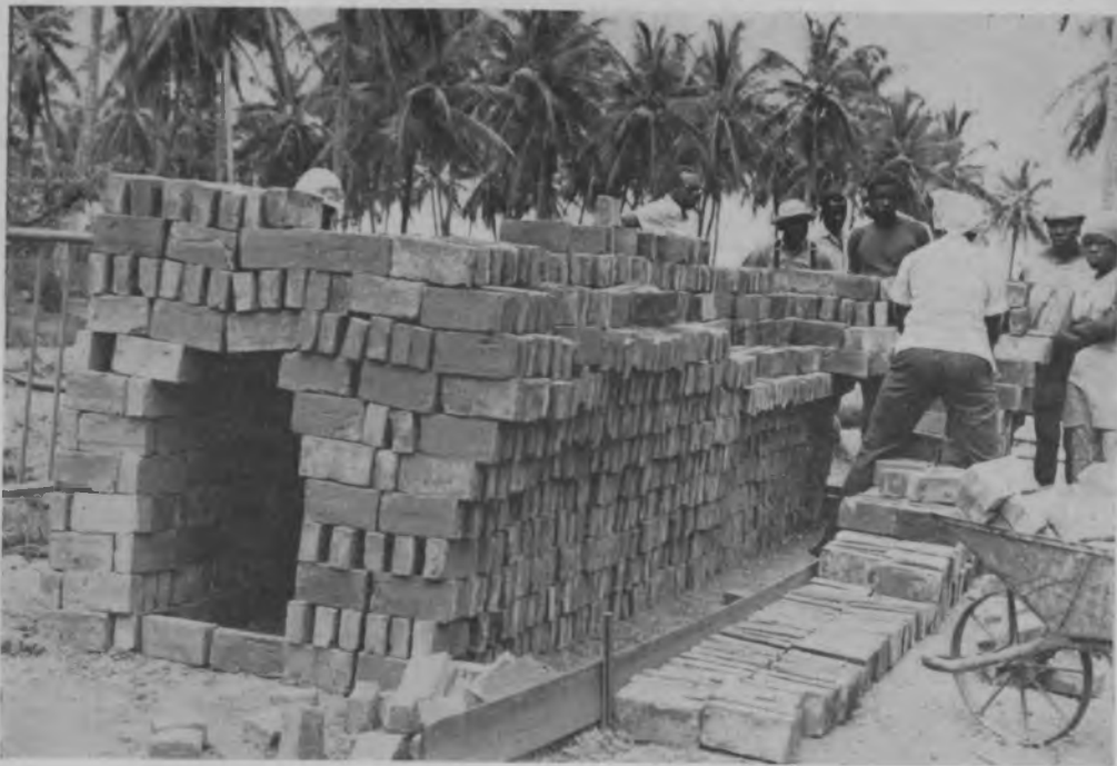
Members of the Victoria Village Co-operative Society manufacturing clay bricks
